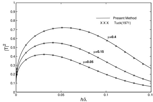
Figure 3:  $|T|^2$  against  $\frac{h}{\lambda}$  for different values of  $\mu$ , and  $\alpha = 0^0$ .
