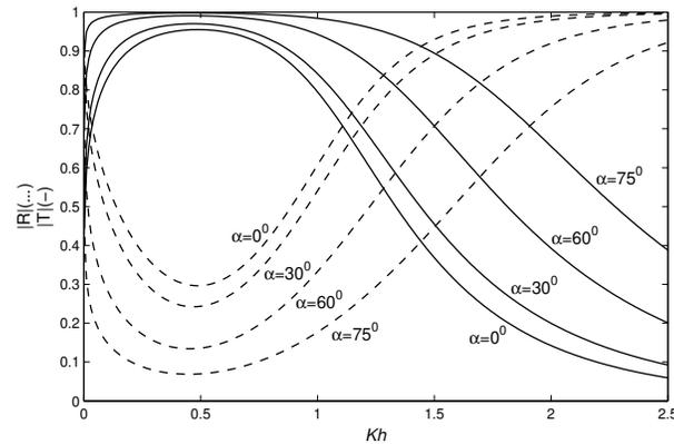
Figure 6:  $|R|(\dots)$  and  $|T|(-)$  against  $Kh$  for different values of  $\alpha$ , and  $\mu = 0.5$
